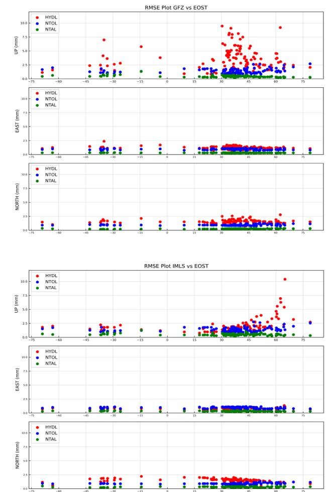
**Figure 2.** RMS values of difference of site displacement due to all non-tidal loading between ESMGFZ and EOST (top) and between IMLS and EOST (bottom). Large RMSE values are mainly observed between 30°N to 65°N for up direction. The RMSE values between two services are maximum for HYDL component, especially in case of ESMGFZ vs EOST.
