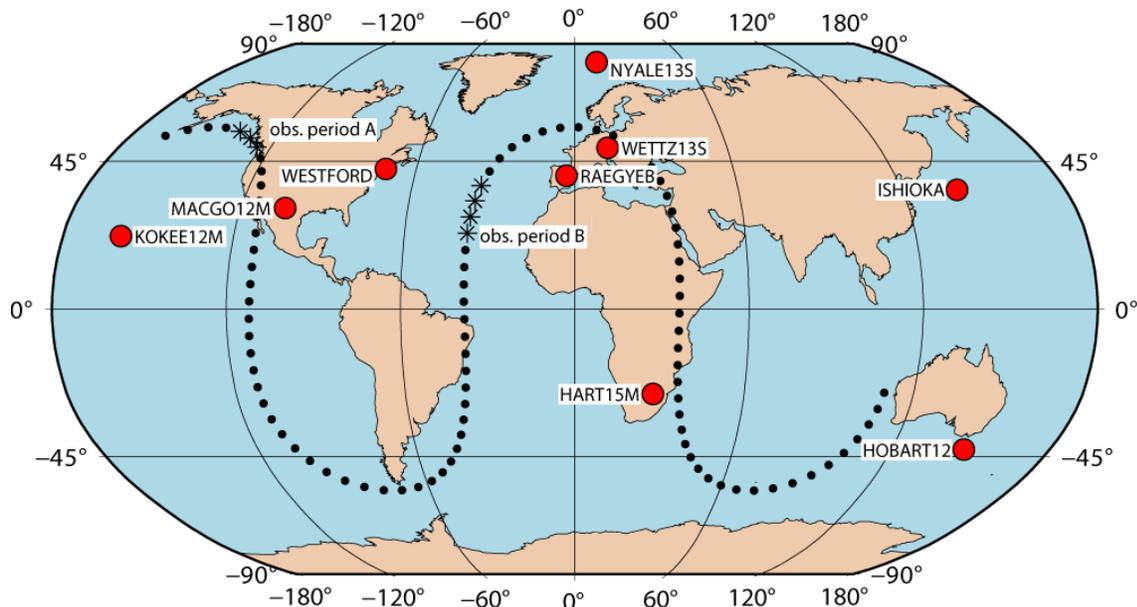
**Fig. 2:** VGOS station network considered in this study and ground track of the satellite GSAT0206 (E30) during 24 hours starting on April 6, 2022, at 00:00:00 UTC. The dots represent the ground track of the satellite at a 15-minute interval. The asterisks mark the positions of the satellite during the observation periods A and B when satellite scans are scheduled.
