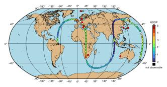
Ground track of GSAT0102 (E12) during the 24-hour IVS-R1978 session on December 21, 2020. The dots represent the position of the satellite over Earth in a ten minute interval color-coded by the values of the UDOP factor. The smaller black dots represent positions where the satellite is not visible from at least two stations.
