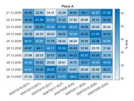
Percentage of time the satellites in Plane A, ordered by their slot number, are observable from at least four stations over a period of 10 days starting on December 21, 2020. A cut-off elevation angle of five degrees is considered.
