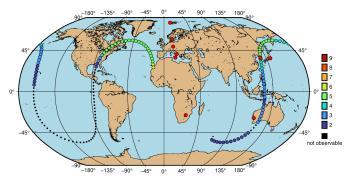
Ground track of GSAT0217 (E27) during the 24-hour IVS-R1978 session on December 21, 2020. The dots represent the position of the satellite over Earth in a ten minute interval color-coded by the number of stations from which the satellite is visible. The smaller black dots represent positions where the satellite is not visible from at least two stations.
