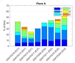
Percentage of time the satellites in Plane A, ordered by their slot number, are observable during the 24-hour IVS-R1978 session on December 21, 2020, color-coded by the number of stations from which the satellite is observable. A cut-off elevation angle of five degrees is considered.
