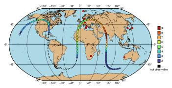
Ground track of GSAT0216 (E25) during the 24-hour IVS-R1978 session on December 21, 2020. The dots represent the position of the satellite over Earth in a ten minute interval color-coded by the number of stations from which the satellite is visible. The smaller black dots represent positions where the satellite is not visible from at least two stations.
