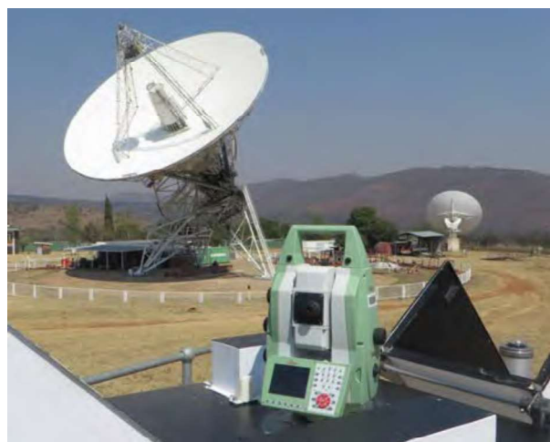
Fig. 1: Short baseline of \sim 113 m between the HartRAO 26 m antenna (left) and the HartRAO 15 m antenna (right), with the Leica MS50 Multistation in the foreground.
