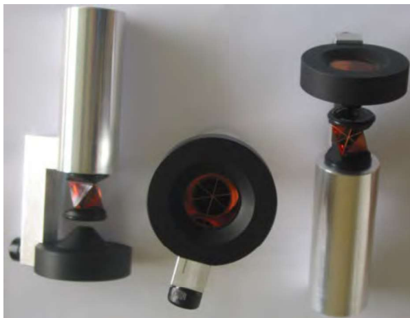
Fig. 3: Targets, consisting of a combination of Leica prisms and custom-made adapters.
