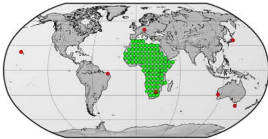
Fig. 2: Investigated network: seven fixed stations (red dots) plus one station with 99 possible positions (green dots)
