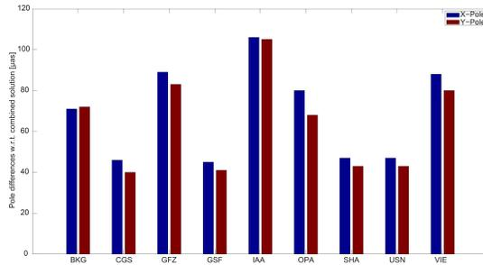
Fig. 3 WRMS of pole residuals w.r.t. the combined solution.
