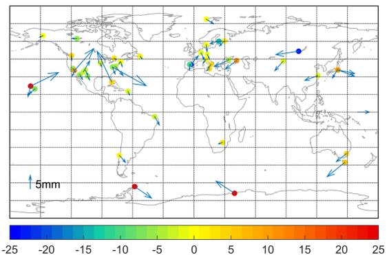
Fig. 8 Position differences between VieTRF2014a and VTRF2008 at epoch 2000.0. Only stations with an RMS of less than 5 mm are shown. The color bar represents the height difference in mm
