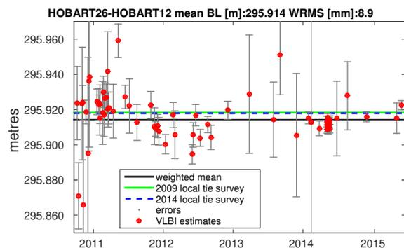
**Fig. 1** The Hobart-Hobart baseline determined of 72 common VLBI sessions. The black line shows the mean calculated baseline length of 295.914 m, which is 4 mm off from the baseline determined in two local tie surveys.
