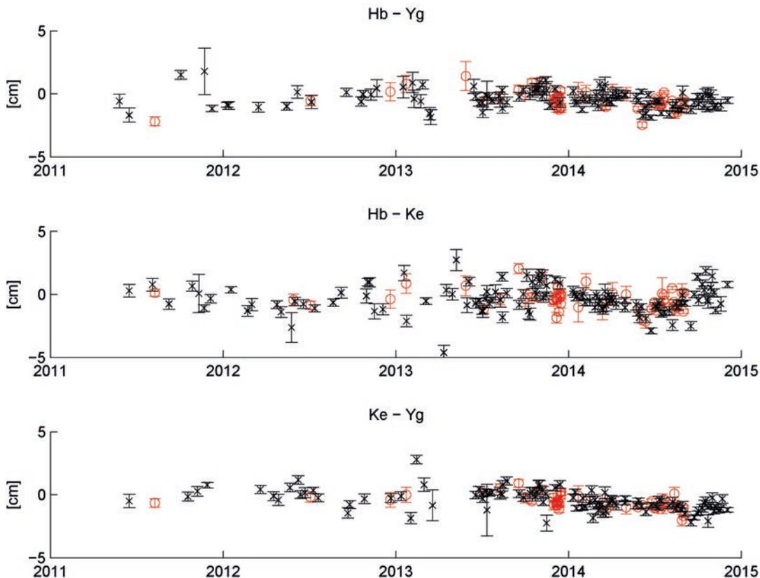
Fig. 5: Estimates and formal errors of AuScope baselines, from IVS-R1 and IVS-R4 sessions (in black), and from AuScope sessions (in red)
