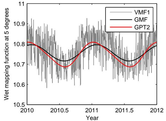
Figure 9: Wet mapping functions at Tsukuba, Japan at 5 degrees elevation
